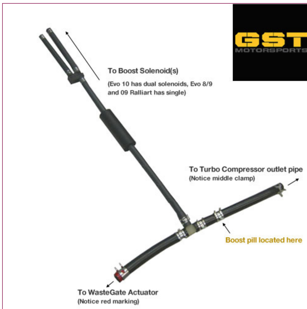
Figure 44: BOOST TUNING – WASTEGATE ACTUATOR HOSE & PILL SETUP, EVO X
