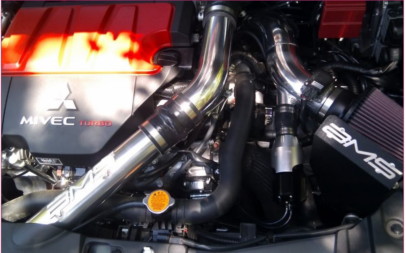
Figure 46: BOOST TUNING – SYNAPSE BOV on EVO X, on AMS intake pipe
