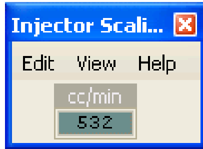
Figure 59: INJECTOR TUNING – INJECTOR SIZE SCALING, RALLIART & EVO X
