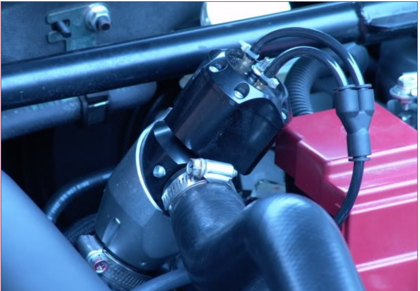
Figure 45: BOOST TUNING – SYNAPSE BOV on EVO X, stock mounting position
