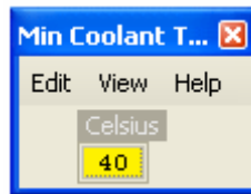
Figure 18: FUEL TUNING – tuned LAMBDA TEMP THRESHOLD
